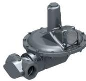
To achieve that task the use of Elster American Meter Series 1800 units that can handle inlet pressures of up to 150 PSI with outlet pressures as low as 3.5" WC are the regulator of choice. Shown in the thumbnail image to the left, these rugged industrial regulators are in service on millions of critical gas regulation applications and are stocked at Meters & Controls.
